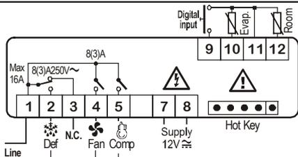
**NOTE:** The compressor relay is 8(3)A or 16(6)A according to the model.
