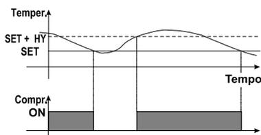
The regulation is performed according to the temperature measured by the thermostat probe with a positive differential from the set point: if the temperature increases and reaches set point plus differential the compressor is started and then turned off when the temperature reaches the set point value again.
