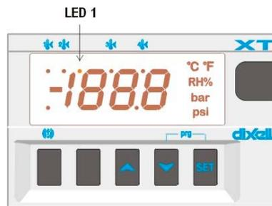
**SET:** To display and modify target set points; in programming mode it selects a parameter or confirm an operation.
