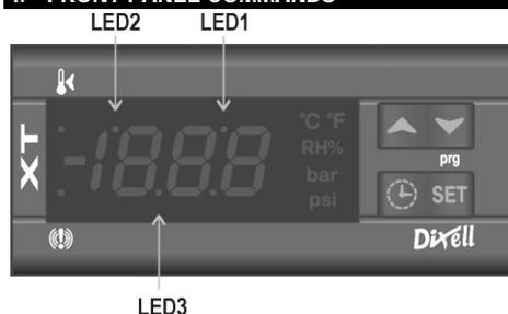
**SET:** To display and modify target set point: in programming mode it selects a parameter or confirm an operation.
