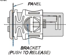
To obtain an IP65 protection grade use the front panel rubber gasket (mod. RG-C).
