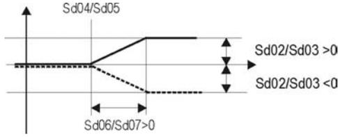
Pb4 probe with negative differential (below)
