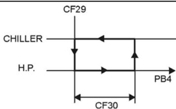
When the temperature value is within the **CF30** range, the changeover is allowed only though keyboard.
